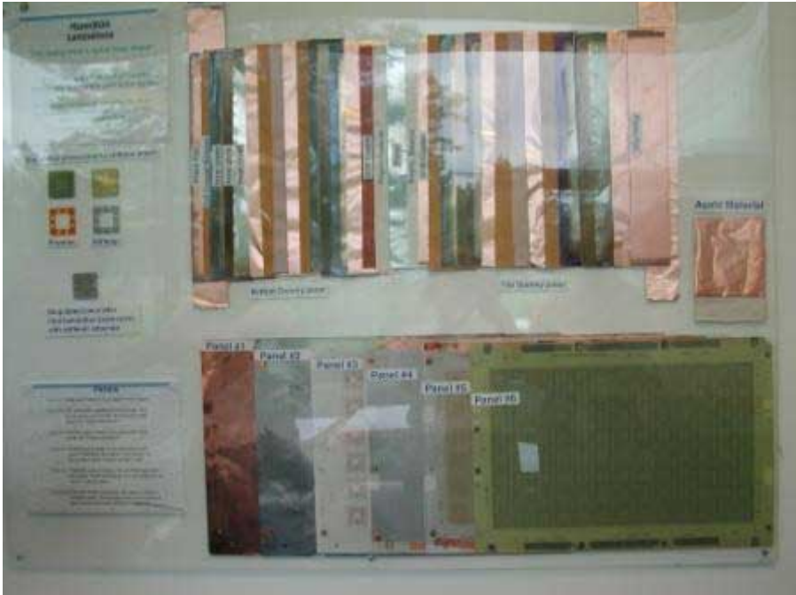
Figure 2. Display of EI's HyperBGA lamination layout diagram of the steps to create a panel that then becomes BGA substrates.
