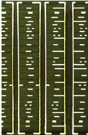
Driclad ® in a 28 layer high reliability server board
